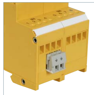
Separate earth connection on the unprotected side of the device. The second slot of the double terminal is intended for connecting the terminal equipment to the equipotential bonding.
