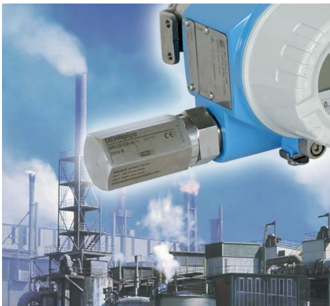
Surge arrester for outdoor use to be screwed onto two-wire field devices. Stainless steel, installation with cable gland up to IP 67.
