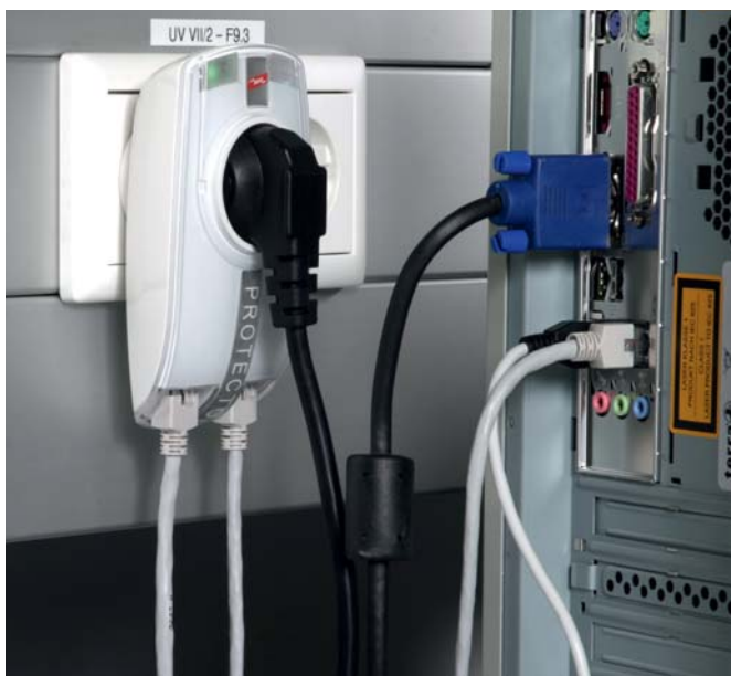
Combined surge protective adapter with visual operating state and fault indication plugged into an earthed socket outlet.
