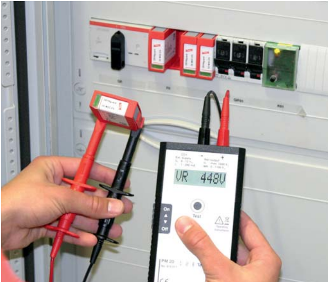
For testing the sparkover voltage of surge arresters. The specimen is connected via the included test leads or special test adapters.
